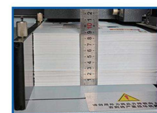
Upper suction air automatic paper feeding paper thickness 90mm
