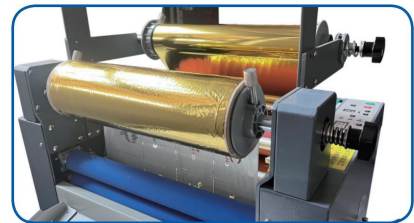
Automatic winding of hot stamping waste
