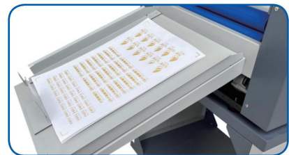
Automatic collection of bronzing finished products
